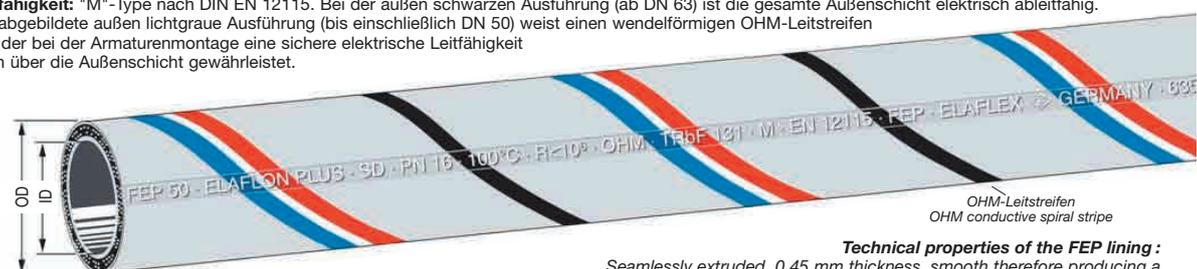
**Electrical conductivity:** "M" - Type acc. to EN 12115. Hoses with black cover (from DN 63) have an entirely electrically dissipative cover. Hoses with grey cover (up to DN 50) have a OHM conductive spiral stripe which guarantees a safe electrical conductivity of the hose assembly after the fittings have been mounted.
